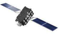
Existing GPS systems can have inaccuracies measured in meters – the Michibiki satellites covering Japan will be accurate down to several centimeters, unlocking the potential of autonomous vehicles within the Japanese market, among other activities reliant on high levels of accuracy.
